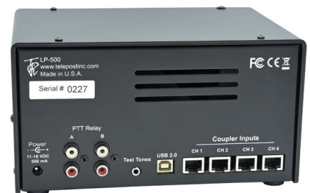
Figure 6 — The LP-500 rear panel with connections for power, PTT relay, test tone output, USB connection to a computer, and four couplers. (Lab tests were performed with LP-500 serial number 0325; see the Lab Notes sidebar.)
