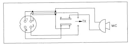
If the microphone to be used is provided with pre-cut leads, they must be revised as ollows:
