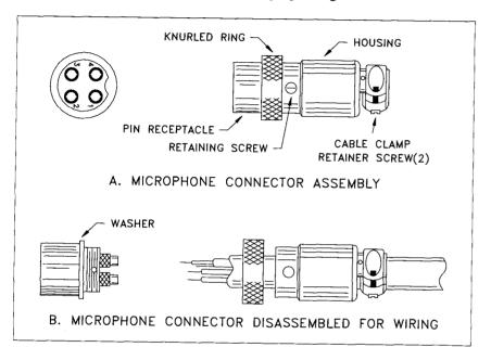
Fig. 2 Microphone plug wiring
