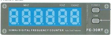
Measures contacted RF signal or TX signal from ant. Range up to 50Mhz, Input Level from 0.1~1V Max.
