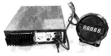
The frequency counter jack has to connect to the SRA-166FB/FC, it will display blue illuminated indicates the frequency of the selected channel. Insert the audio plug SRA-166FB/FC into the public address speaker or external speaker transceiver , so you can hear the sound.
