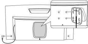
Dock. Push the antenna over the mounting brackets and then slide the antenna down slightly to secure it in place. Last, open the antenna clamshell so that the top of the antenna is facing the sky.
