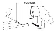
To mount the antenna, you will need four screws (sold separately) with a 1/4" head (e.g., a #4 screw), and that are suitable for the material onto which you are affixing the antenna, (e.g., wood, metal, etc.). The screws should be spaced 1-3/8" apart horizontally and 1-1/8" vertically. Refer to the "Indoor/Outdoor Home Antenna Template" on page 50.
