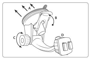
Step 3. Adjust the angle and rotation of the pedestal head by loosening the swivel-tightening ring (D).
