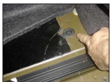
Remove the rubber body grommet towards the back of the floor as indicated.
