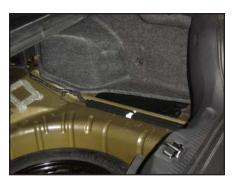
**STEP 2**Remove the trunk floor covering.
