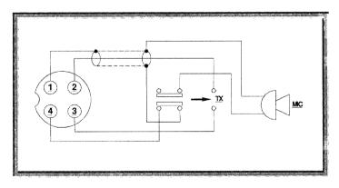
Transceiver Microphone Schematic Diagram
