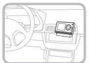
B. Some vents have recessed louvers. If yours are recessed, remove the regular vent clamps and install the extended vent clamps.
