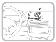
B. Orient the adhesive foot so that Onyx is easily accessible. Loosen the knob and adjust the adhesive foot to position 1 or 2, and then tighten it.
