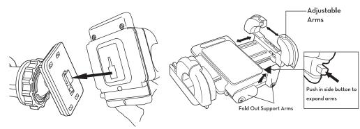
Place the Grip-It over the T-Notch and slide it down securing it to the mount.
