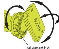
Note: Do not overtighten the Adjustment Nut.
