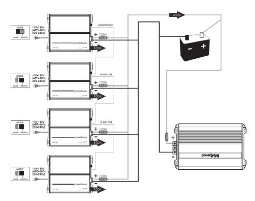
WARNING: Do not overload AC power outlets to avoid danger of electric shock and fire. A minimum current of 20A per APS-100 will be required. Avoid connecting multiple power supplies to a single AC outlet using power strips.
