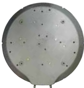
Bottom of antenna, eyelet removed
